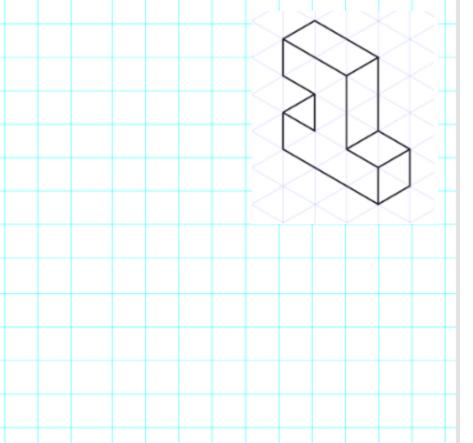
**Orthographic Drawing** The **definition** of an **orthographic** projection is a two-dimensional **drawing** of a three-dimensional object, using two or more additional **drawings** to show additional views of the object. Draw the top front and right views of the Isometric drawing.
