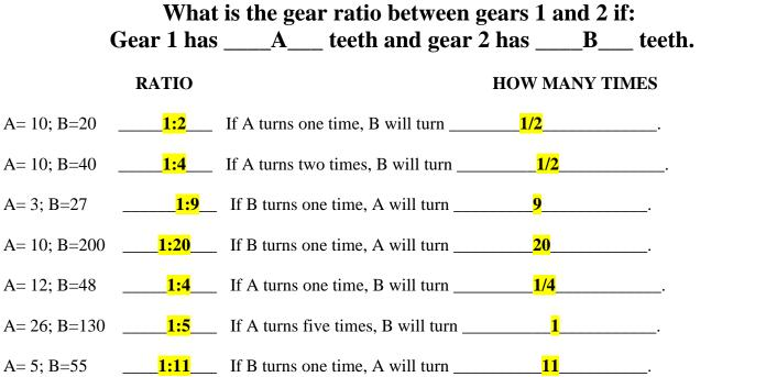
In Gear-trains with multiple gears the ratio will change from set to set, but ends as a ratio from the first to the last.
