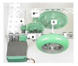
*Example:* A has 10 teeth; B has 40 teeth; the ratio for the A:B is 40:10, or 4:1.  $B^{**}$  has 10 teeth; C has 50; the ratio for  $B^{**}$ :C is 50:10, or 5:1. Multiply 5:1 x 4:1 and you have 20:1
